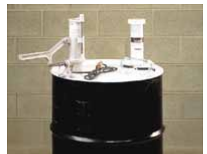
This device is used to drain all residual aerosol and product from aerosol cans, so that the empty metal cans can be compacted and recycled.
